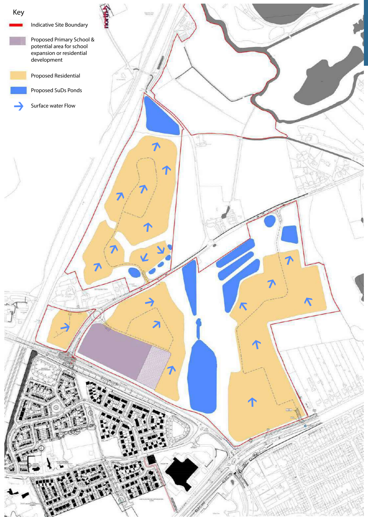
PROPOSED SuDS & SURFACE WATER FLOW PLAN
